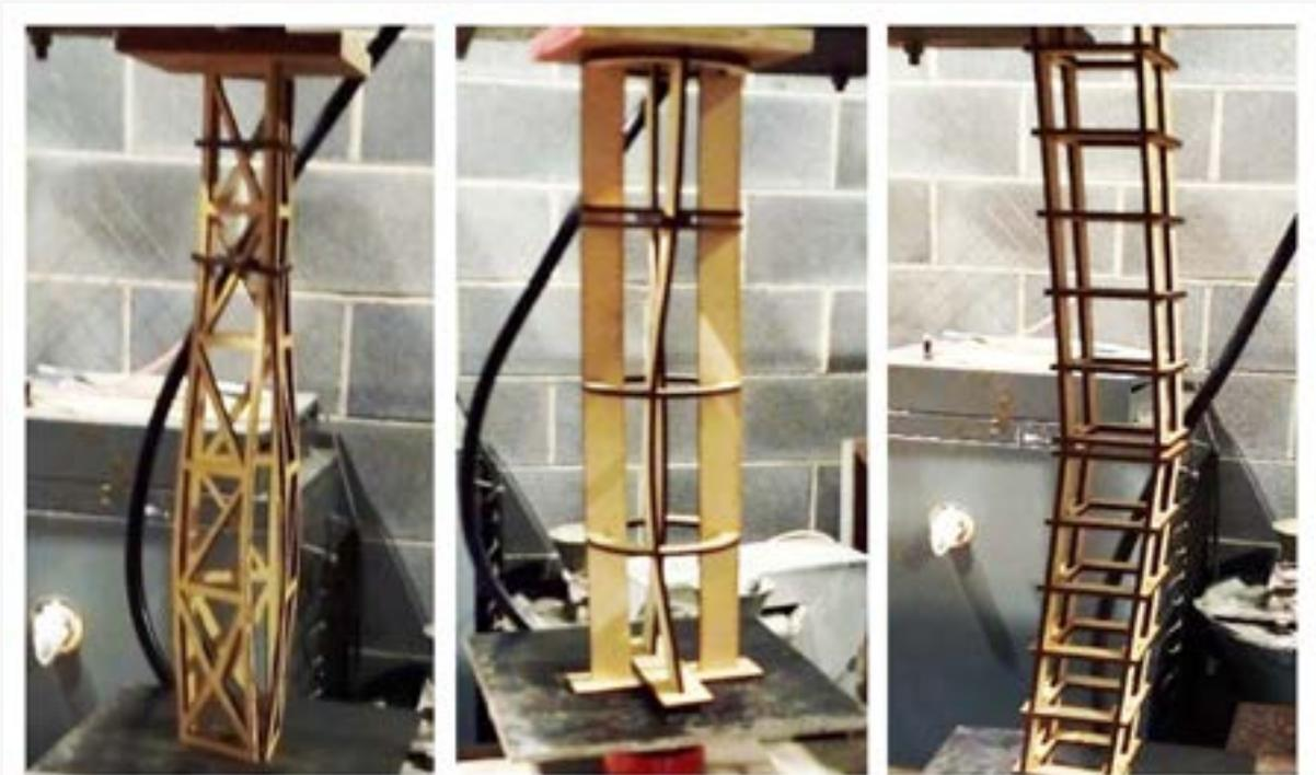
**Figure 10.** Photographs of laser cut model towers being load tested in Week 12 in the Civil Engineering Laboratory (from 2019/20)
