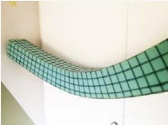
**Figure 5. Foam beam bending model with gridlines to indicate compression and bending stresses**
